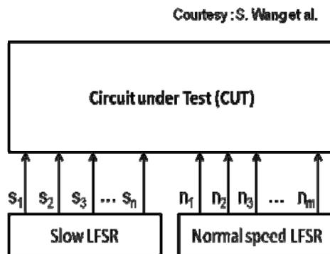
Figure 5 Dual speed LFSR (DS-LFSR)
