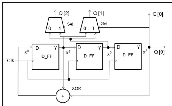
Figure 4 Three stage Bit swapping LFSR
