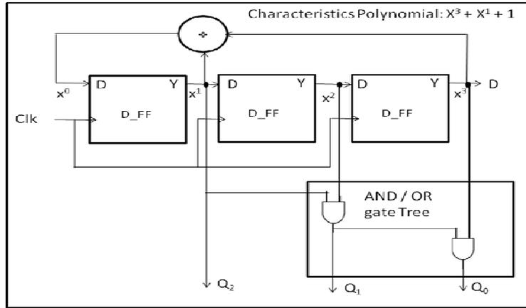
Figure 6 Weighted LFSR (3- Bit)
