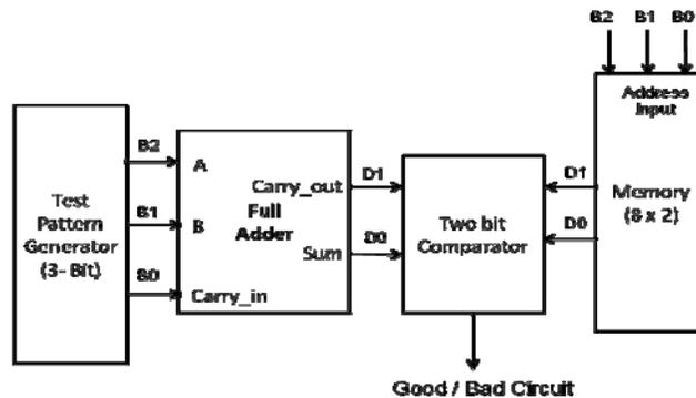
Figure1. Test environment for Full adder circuit
