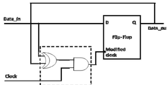
Figure 3. Gated clock D flip-flop
