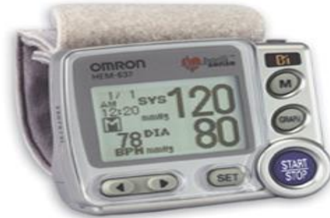
Figure 6: Tilt sensing example, Omron Wrist blood pressure monitor with advanced positioning sensor
