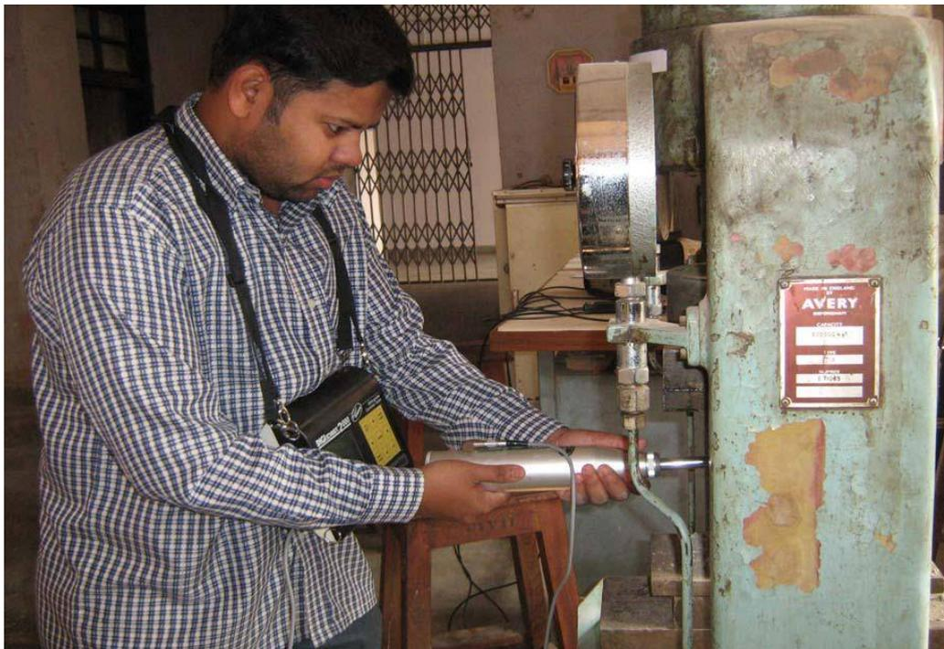
Fig.5.2 Rebound Hammer Testing of a Specimen
