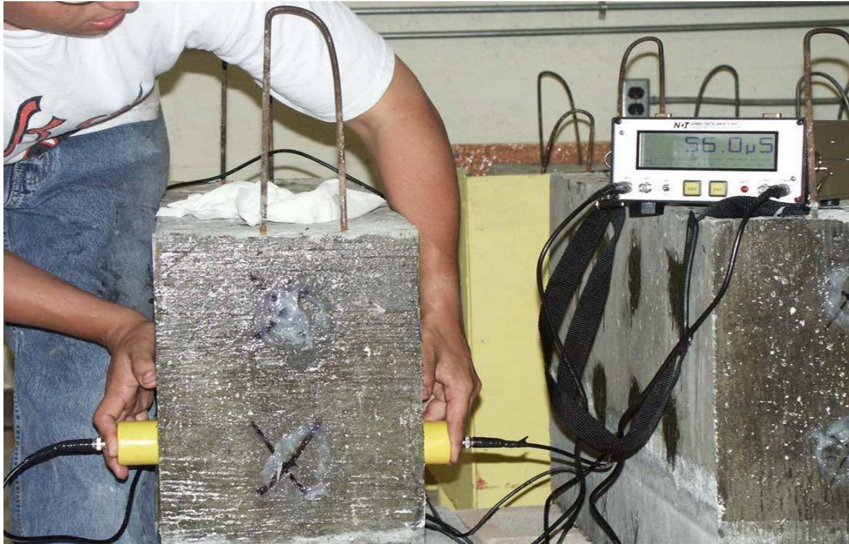
Fig.4.3 Testing of a beam by USPV Tester
