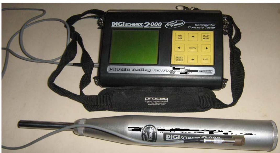
Fig.5.1 Components of a Rebound Hammer used in the Project
